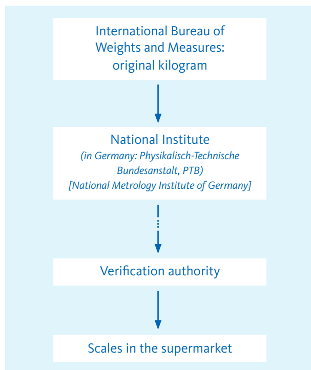
Fig. 1 Traceability chain for supermarket scales
