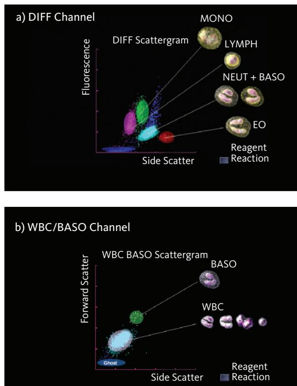
**Fig. 3** Sysmex X-Class analyser scattergrams. a) Differential scattergram: fluorescence which is a measure of RNA/DNA content of cells is represented on the Y axis and cell complexity or side scatter is represented on the X axis. b) WBC/BASO channel – this channel, present on the XT and XE analyser, utilises a chemical reaction which keeps basophils intact to separate them from the remaining white blood cells on the basis of forward scatter (Y axis) and side scatter (X axis).
