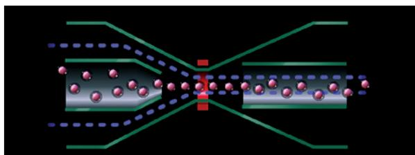
Fig. 1 Impedance principle with hydrodynamic focusing.
